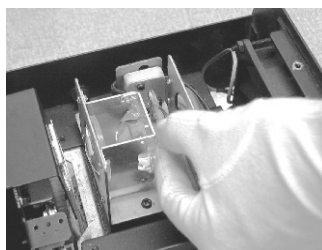
Installing the Lamp (EHJ)
