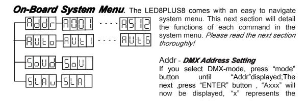
displayed address. Press the UP or DOWN buttons to find your desired address. Then press "ENTER" botton for three second; It will be set;
